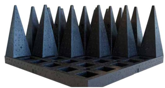
Polypropylene (pp) based hybrid pyramid absorber is a product that is optimalized to be used in a EMC chamber and is available in a different range of sizes. When used with ferrite tile 3600, the 3700 series has a broadband operating frequency range starting from 30 MHz and up to 40 GHz.
